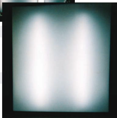
FL20×2 units; Pitch: 250mm; Milk translucent: Mitsubishi Rayon's #430, 3mm t; Signboard thickness: 90mm
