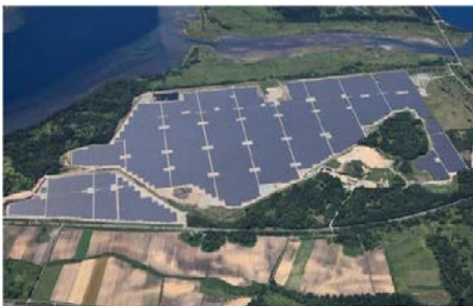
Rokkasho Solar Park First renewable energy project in Japan to use 154kV
