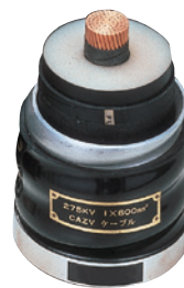
275 kV cross-linked polyethylene insulated, aluminum sheathed, PVC outer sheathed cable
