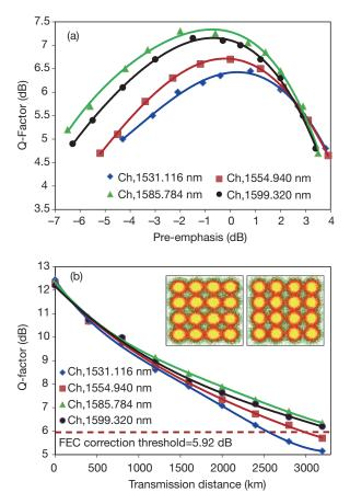
Figure 8 Performance vs transmission distance, inset are the recovered constellations for x- and y-polarization of the channel 1554.94 after 2400 km.
