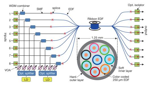
Figure 4 Schematic diagram of 1x8 arrayed EDFA, inset: schematic of 8 EDF ribbon; (b) Measured gain and gain deviation of individual EDFA in arrayed EDFA.
