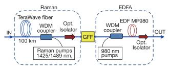
Figure 6 Schematic diagram of complementary Raman/EDFA for 100 km TeraWave fiber span.
