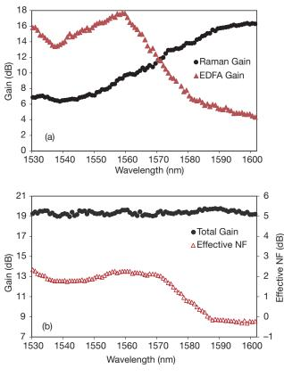
Figure 7 (a) Measured EDFA gain and Raman gain from the complementary Raman/EDFA, (b) measured total gain w/ GFF and effective NF.
