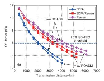
Figure 3 Q<sup>2</sup> factor versus transmission distance of the 10-channel 256 Gb/s PDM-16QAM system using the three different amplification schemes without (solid curves) and with ROADMs (dashed curves) with 50 GHz channel spacing. Optimum launch powers are used.
