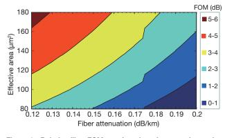
Figure 1 Relative fiber FOM as a function of attenuation and effective area for 80 km spans in long haul systems.
