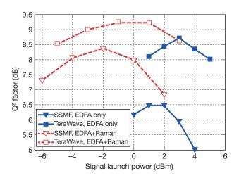
Figure 2 Measured Q<sup>2</sup> vs launch powers of 485 Gb/s CO-OFDM signal transmission over 1600 km of TeraWave and SSMF<sup>3</sup>.
