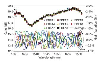
Figure 5 Measured gain and gain deviation of individual EDFA in arrayed EDFA.
