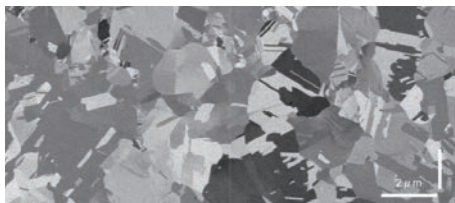
図5 銅箔の断面結晶組織 X-section crystal structure of copper foil.
