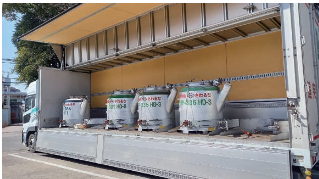
図8 溶湯搬送 2) Molten metal transfer.
