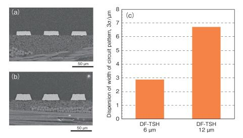
Figure 2 Fine pattern formation on  $L\&S = 30/30 \ \mu m$  by the Subtractive process.
