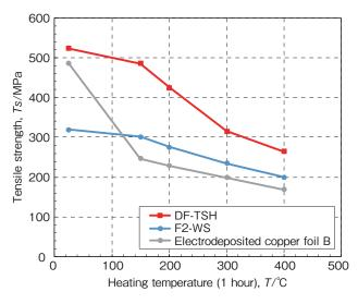
Figure 3 Thermal stability of DF-TSH compared with other electrodeposited copper foils.
