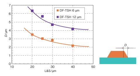
Figure 1 Effect of the copper foil thickness for pattern trailing length D by the Subtractive process.
