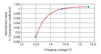
Figure 9 Normalized SOC at full charge detection against various charging voltage.
