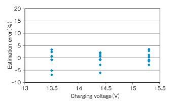
Figure 11 Error of the estimated full charge when considering the charging voltage.
