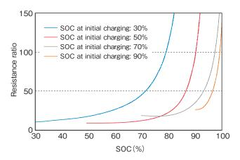
Figure 6 Difference of the relation between the resistance ratio and the SOC caused by difference of SOC at initial charging.
