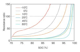
Figure 5 Difference of the relation between the resistance ratio and the SOC caused by the different temperature.
