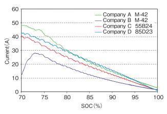
Figure 2 Relation between the charging current and the SOC.
