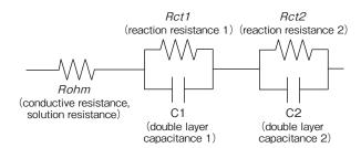
Figure 3 An example of the equivalent circuit model.
