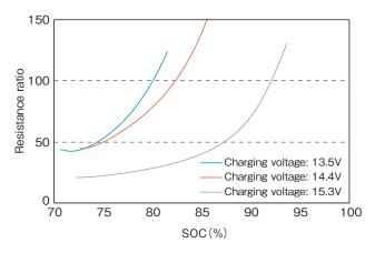
Figure 7 Difference of the relation between the resistance ratio and the SOC caused by difference of charging voltage.
