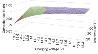
Figure 10 A 3-dimensional curved surface of correction coefficient vs. charging voltage and temperature.
