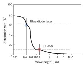
Figure 2 Light absorption rate for copper.
