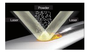
Figure 3 LMD using a multi-beam method.
