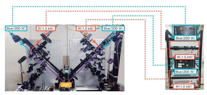
Figure 10 Setup photograph of a hybrid laser irradiation optical system that combines a blue diode laser and a near-infrared fiber laser.
