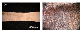
Figure 14 Bead-on welding experiment results using a multibeam processing head (output 1,000 W). (a) Cross-sectional photograph in the direction perpendicular to the scanning direction of the laser focused spot (b) Surface photograph
