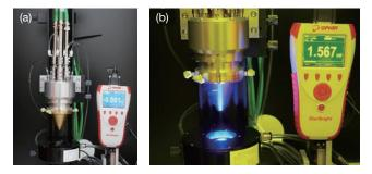
Figure 12 Multi-beam processing head using three 500 W blue diode lasers has been developed. (a) Processing head (b) Laser output
