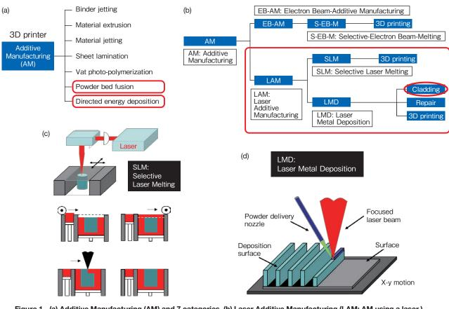
Figure 1 (a) Additive Manufacturing (AM) and 7 categories, (b) Laser Additive Manufacturing (LAM: AM using a laser.), (c) Selective Laser Melting (SLM: Powder bed fusion method using a laser.), (d) Laser Metal Deposition (LMD: Directed energy deposition method using a laser.)
