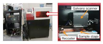
Figure 7 External appearance photograph of a SLM method 3D printer equipped with a blue diode laser.
