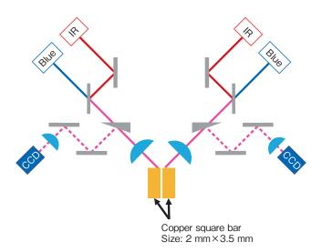
Figure 9 Setup diagram of a hybrid laser irradiation optical system that combines a blue diode laser and a near-infrared fiber laser.
