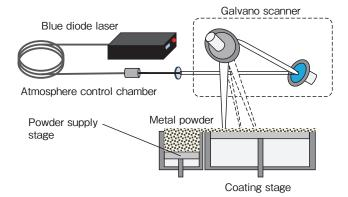
Figure 6 Schematic diagram of a SLM method 3D printer equipped with a blue diode laser.
