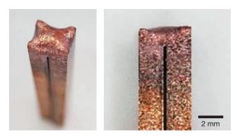
Figure 11 High-speed welding for a pure copper square wire using a hybrid laser system that combines a blue diode laser and a near-infrared fiber laser.
