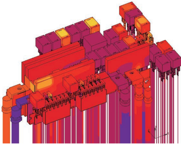
Figure 12 3D contour view of the R/B thermal analysis.
