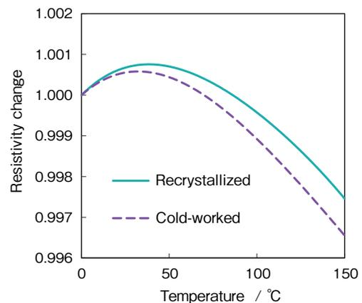
**Figure 11** Relationship between the resistivity change and the temperature in the recrystallized and the cold-worked Alloy-1.
