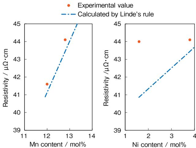
**Figure 5** Relationship between the resistivity and (a) Mn content in Cu-xMn-3.8Ni alloy, (b) Ni content in Cu-12.8Mn-yNi alloy.
