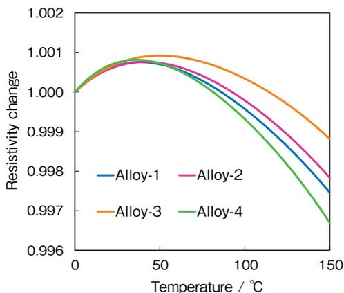
**Figure 6** Relationship between the resistivity change and the temperature in each alloy.
