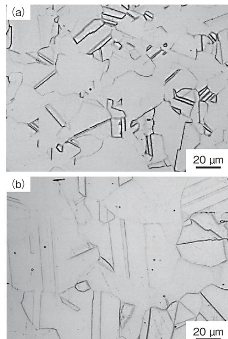
**Figure 7** Microstructures of Alloy-1 annealed for (a)  $3.6 \times 10^3$  s, (b)  $2.6 \times 10^5$  s.
