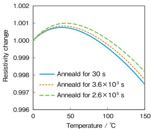
**Figure 9** Relationship between the resistivity change and the temperature in Alloy-1 annealed for each time.
