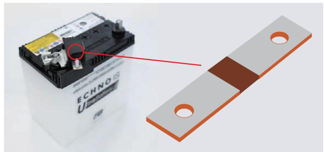
Figure 2 Example of a bus-bar type shunt resistor application.
