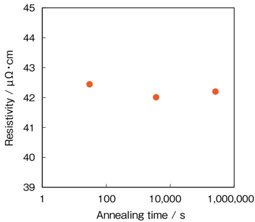
**Figure 8** Relationship between the resistivity at 20°C and the annealing time at 600°C in Alloy-1.
