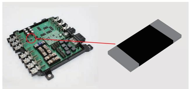
Figure 1 Example of a chip resistor application.
