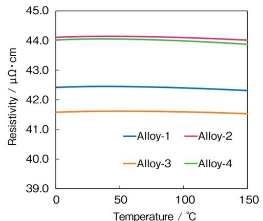
**Figure 4** Relationship between the resistivity and the temperature of each alloy.
