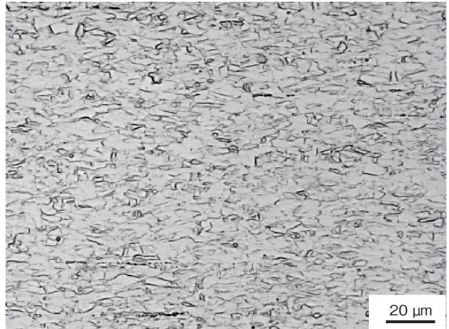
**Figure 10** Microstructure of the cold-worked Alloy-1.
