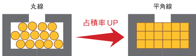
図10 丸線と平角線のモータ内占有率差 Difference in occupancy rate between round wires and rectangular wires in the motor.
