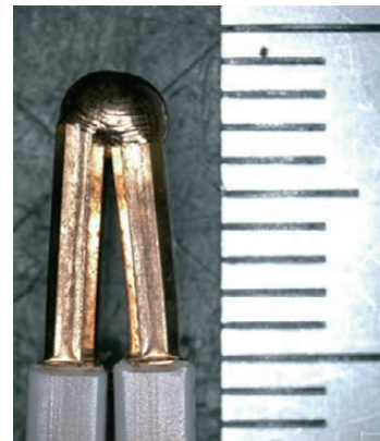
図13 剥離長8 mmのPEEK被覆付き平角銅線ヘアピン溶接部 Optical images of hairpin welding of PEEK resin coated rectangular copper wires with 8 mm stripping length.
