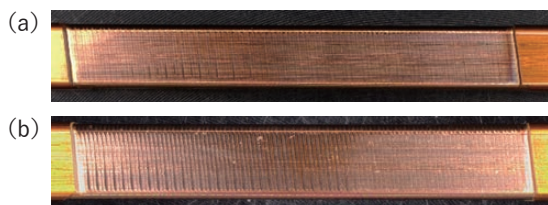
図4 被膜除去後のサンプル (a) BR0400両面照射, (b) BR0700両面照射 Surface states after removing PI coating of copper rectangular magnet wire, (a) by BR0400, and (b) by BR0700, each by both side laser irradiations.
