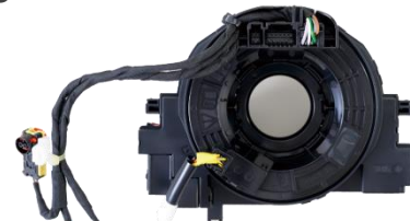
SRC (Steering roll connector)
