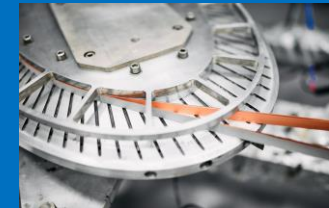
High temperature superconducting magnet coil undergoing testing (Image provided by Tokamak Energy)
