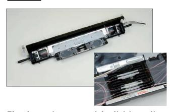
The closure integrates eight-division splitter function with WDM filter function using planar lightwave circuit (PLC) technology only, facilitating configuration of one-core three-wave FTTH system.
