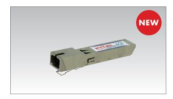
This is an SFP-type ultra compact E-PON ONU compliant with the IEEE802.3ah.
