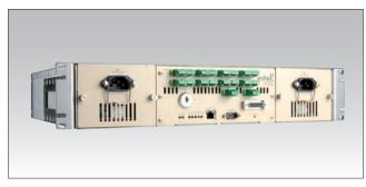
SNMP manageable multiple port optical amplifiers for FTTH video distribution. Selectable are the port number (4, 8, 16 or 32) and the optical output power (11.5, 13, 16 or 20dBm/port).
