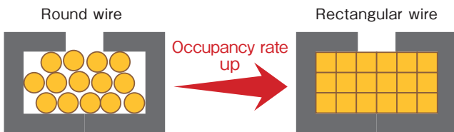
Figure 10 Difference of compactness between round wires and rectangular wires in the motor.
