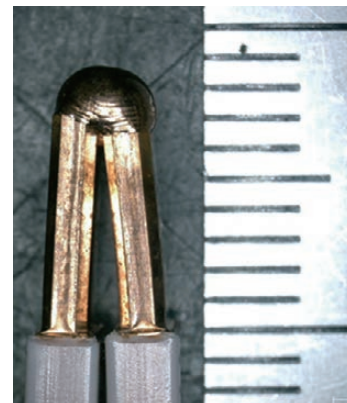
Figure 13 Optical image of hairpin welding of PEEK resin coated rectangular wires with a stripping length of 8 mm.
