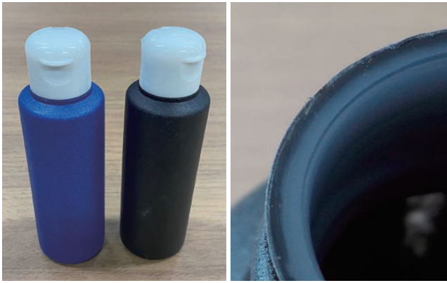
Figure 12 Multilayer bottle (Blow moulded; Outer layer is made from multilayer film waste from Furukawa Electric and beverage cartons. Inner layer is made of PE).
