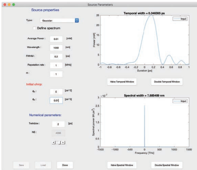
Figure 2 Setting dialogue of the light source. Graphs immediately show the effect of changing any parameter of the source properties in the temporal as well as in the spectral space.
