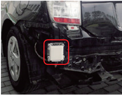
Figure 1 Radar installed inside of the bumper.
